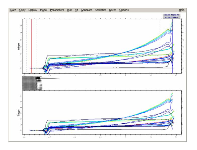
Set the meniscus by dragging the red line to the proper position and hit confirm. Do the same for the bottom and the data limits.
