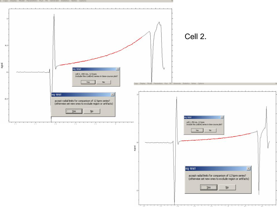
A plot of rms difference over time will be displayed comparing each scan with the previous scan. Here also, the rms difference is unchanged between the last 2 time points. The scans are in equilibrium.
