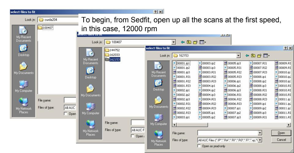
Then, open up all the Interference scans for all the cells in the run.
